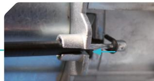
The declutching system acts directly on the reducer. Thus it makes the motor totally free and allows the curtain to be manually and effortlessly operated in case of power failure.
