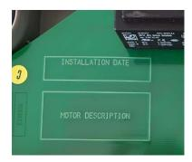
A place is reserved in the box to note the date of installation, as well as a second to paste the removable motor label.
