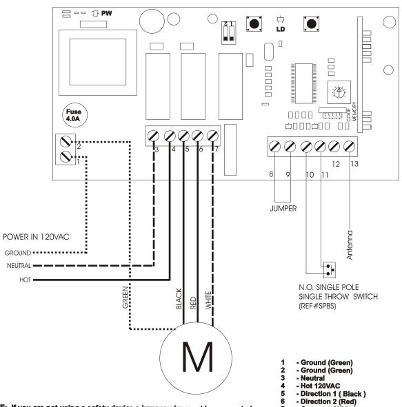
\* NOTE: If you are not using a safety device a jumper wire must be connected to terminals 8 & 9.
